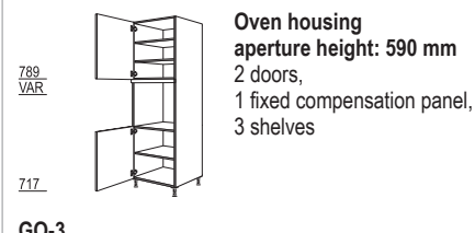
Oven housing aperture height: 590 mm 2 doors, 1 fixed compensation panel, 1 drawer, 3 shelves
