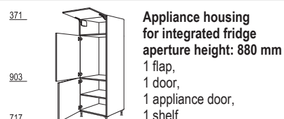
Appliance housing for integrated fridge aperture height: 880 mm 1 door, 1 shelf, 1 appliance door, 2 pull-outs
