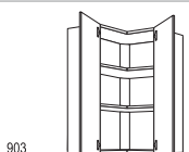
Corner wall unit 2 doors with 165° hinges, 2 shelves, hinged side = first door to be opened
